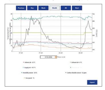
An experiment has been conducted in our offices, to understand CO<sub>2</sub> levels at different times and the impact an MVHR system with and without CO<sub>2</sub> sensor will have upon CO<sub>2</sub> levels.
