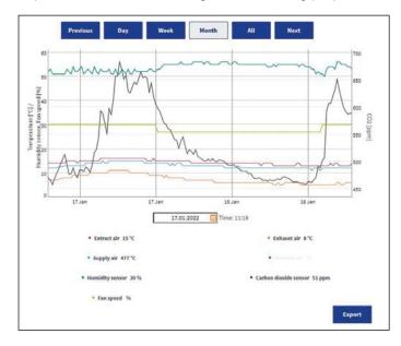
An experiment has been conducted in our offices, to understand  $CO_2$  levels at different times and the impact an MVHR system with and without  $CO_2$  sensor will have upon  $CO_2$  levels.
