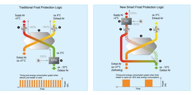
On the traditional frost protection method, the outdoor air is pre-heated before passing through the heat exchanger. This way the unit could still provide balanced ventilation even when the frost protection was on. However, the electric heater kicks in intermittently hence consumes more energy than needed.
