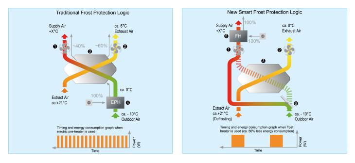
On the traditional frost protection method, the outdoor air is pre-heated before passing through the heat exchanger. This way the unit could still provide balanced ventilation even when the frost protection was on. However, the electric heater kicks in intermittently hence consumes more energy than needed.
