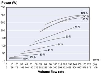
Input power (total) (W) SFP = Air flow (max) (dm<sup>3</sup>/s)
