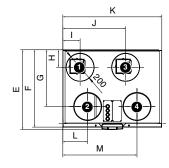
Duct outlets, model L Inner diameter of female outlet collar ø 160 mm 1. Exhaust air out 2. Outdoor air to unit 3. Supply air to dwelling 4. Extract air from dwelling to unit 5. Condensate drain
