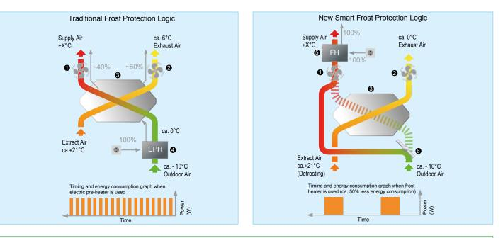
On the traditional frost protection method, the outdoor air is pre-heated before passing through the heat exchanger. This way the unit could still provide balanced ventilation even when the frost protection was on. However, the electric heater kicks in intermittently hence consumes more energy than needed.
