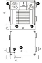
K1. Condensate drain for wall/floor-standing position
