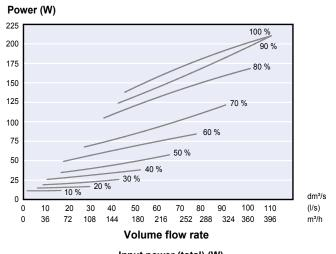
SFP = Input power (total) (W) Air flow (max) (dm<sup>3</sup>/s)
