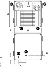
K1. Condensate drain for wall/floor-standing position K2. Condensate drain for under ceiling position
