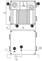
K1. Condensate drain for wall/floor-standing position
